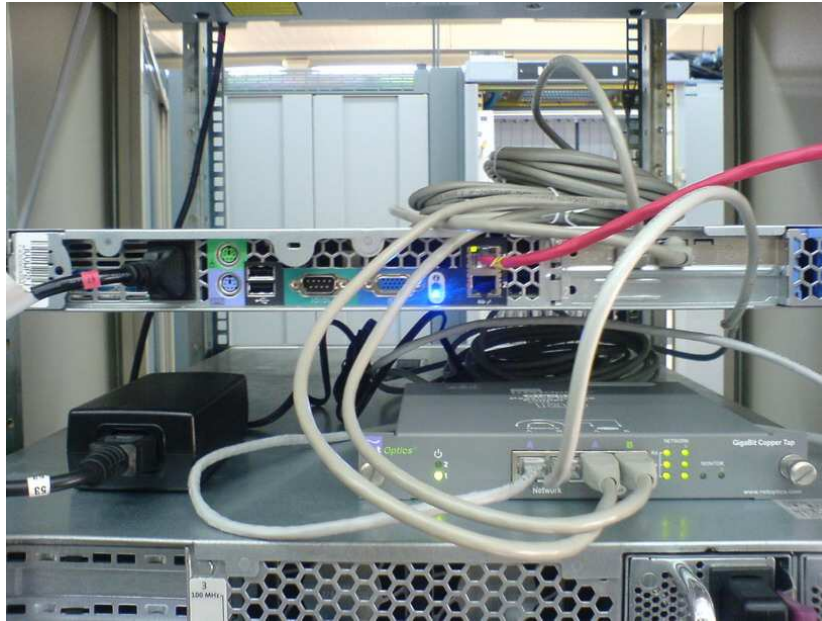
Figure 3.6: The LOBSTER sensor at the Cretan School Network. Note the Gigabit Ethernet Tap used for traffic mirroring under the sensor's 1U server.
