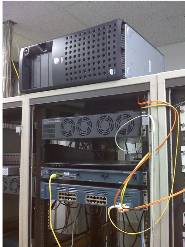
Figure 2.7: FORTH's main LOBSTER sensor. The sensor monitors all traffic between FORTH's campus and the Internet.
