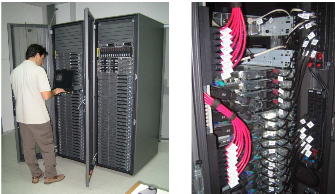
Figure 2.8: FORTH's GRID cluster. One of the 60 nodes is actually a LOBSTER sensor that monitors the traffic of the whole cluster.
