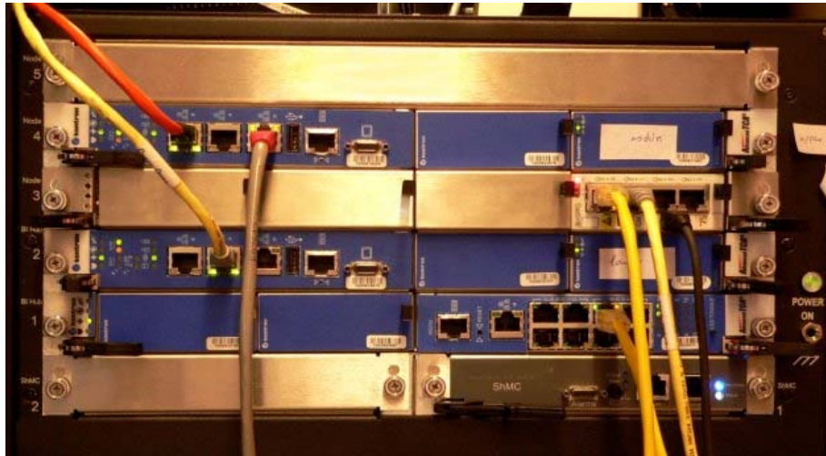
Figure 1 LOBSTER sensor in Alcatel-Lucent lab is embedded in an AdvancedTCA shelf
